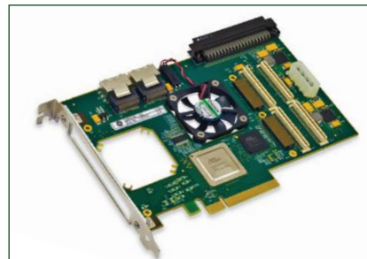
Figure 1 | Short form factor PMC carrier card for PCI applications from GE Intelligent Platforms
